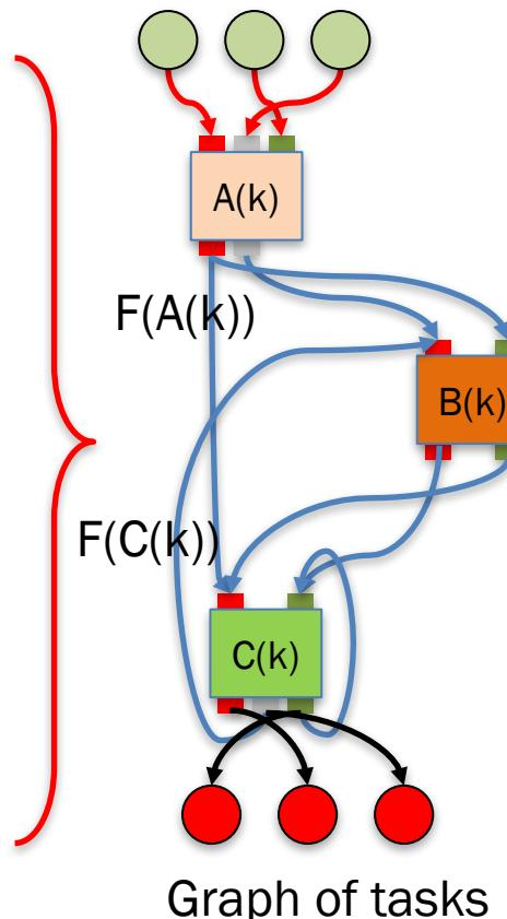
= a **data centric** programming environment based on asynchronous tasks executing on a heterogeneous distributed environment
