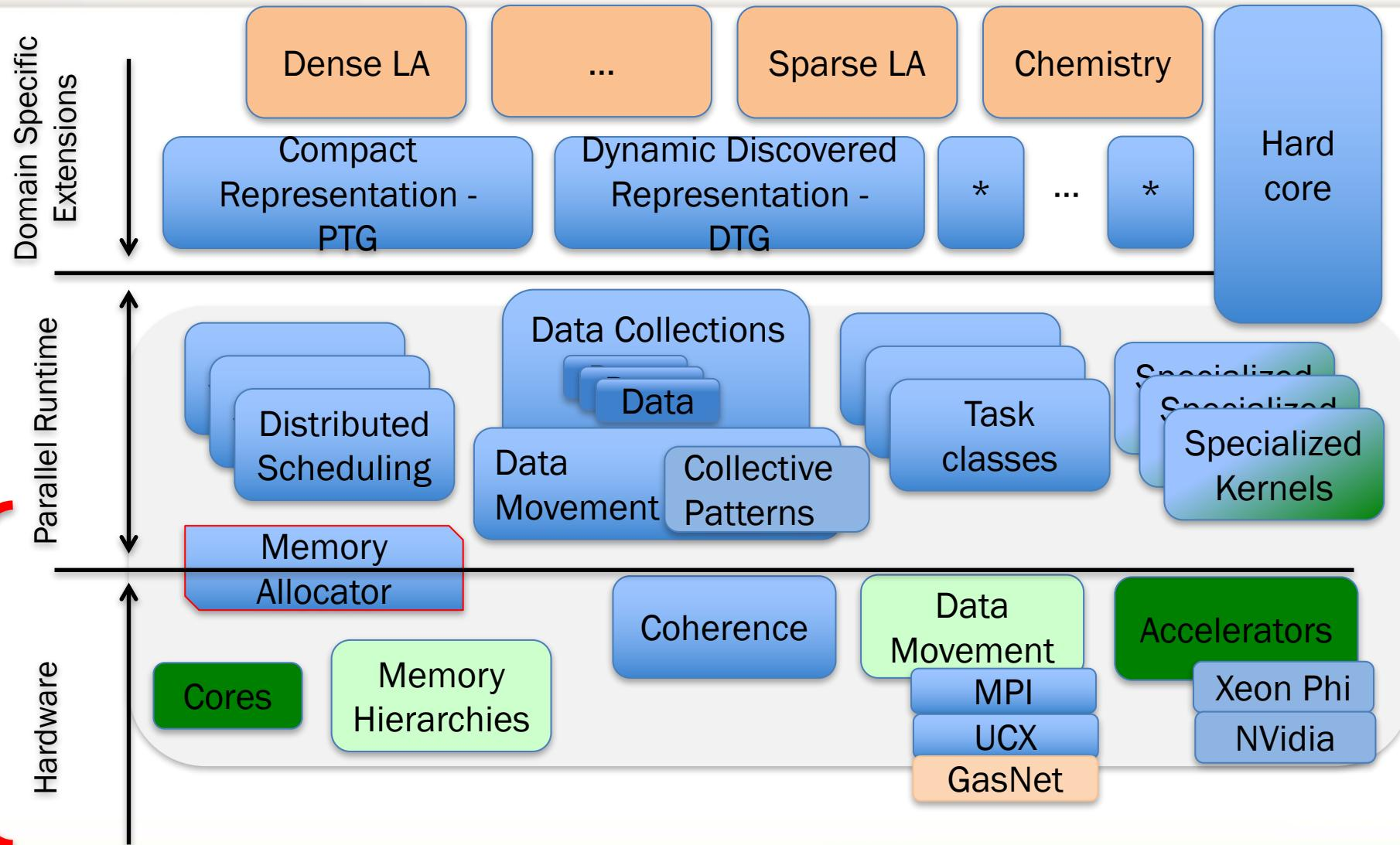
Software design based on Modular Component Architecture (MCA) of Open MPI.
